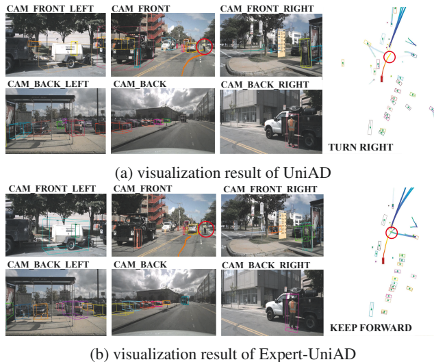
Figure 3: ExpertAD recovery visualization. (a) UniAD misses a traffic officer on the right, leading the vehicle to drift toward them. (b) Expert-UniAD detects the officer, adjusts the trajectory, and completes the lane change safely.
